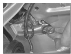
7.7a Release the front direction indicator light retaining spring from its body location . . .
